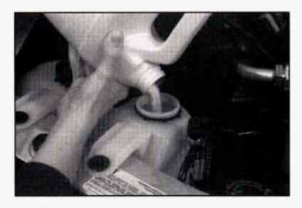
4. Then fill the coolant recovery tank to ADD.
